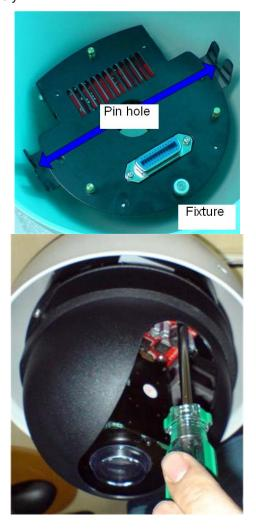
8. Follow anti-clockwise to fix the hemisphere cover onto speed dome.
